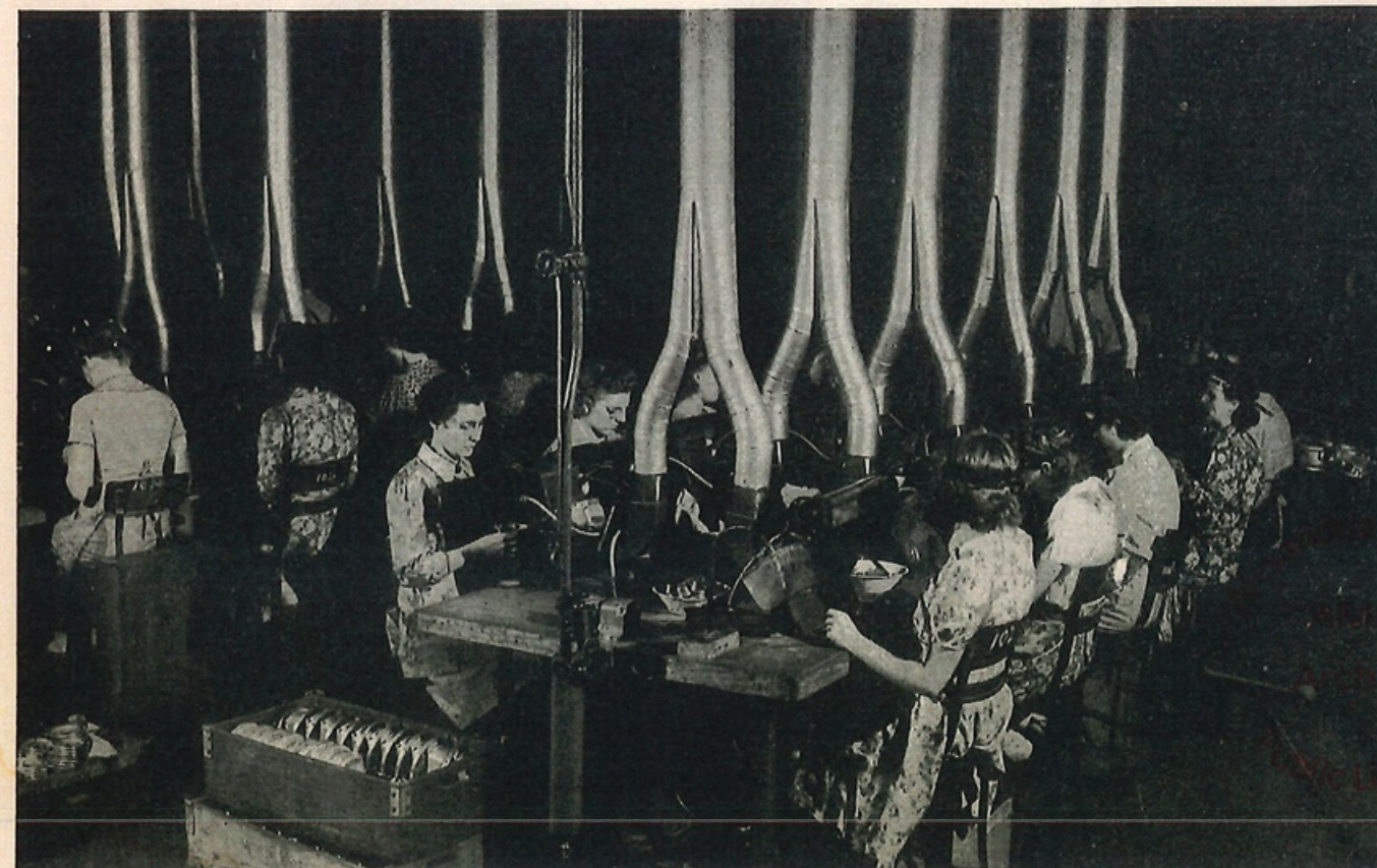
Removing burrs from magneto housings at Delco-Remy. This is a simple operation for which girl workers can be trained in a short time.
